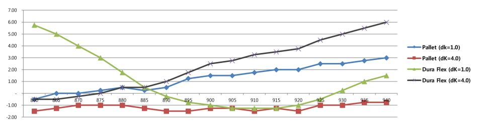
•Pallet, only for non-metal application, reads 6.0 meters on low dielectric materials (dK\*=1) in EU frequency band, whereas 7 meters on high dielectric materials (dK=4) in both EU and US frequency band, all across global band. Pallet reads a little shorter than Dura Flex, but in high dielectric environments, reads longer than Dura Flex. \*dK (dielectric constant)
